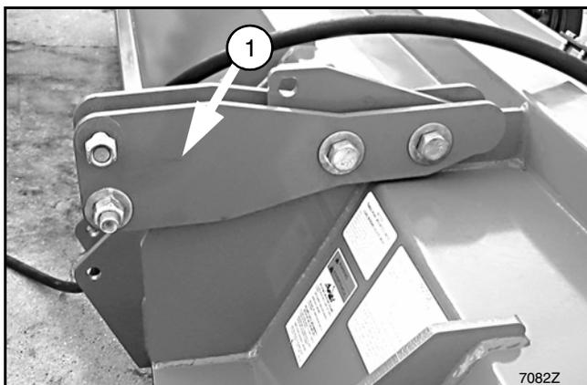
**Figura 42.** Haste flutuante superior instalada
